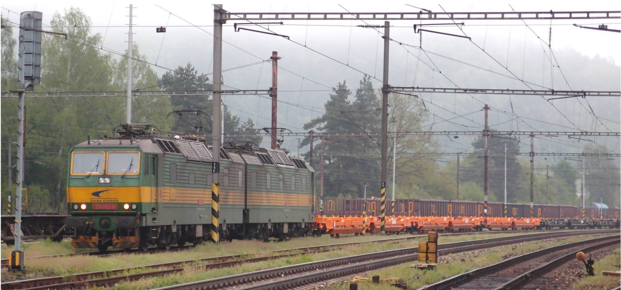
Figure 2: Freight train waiting at Margecany station with most common freight double-section loco (class 131) used on Slovak (and partly Moravian) infrastructure belonging to CS corridor, Photo: J. Ilík
